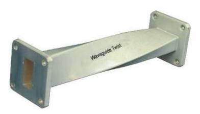
A twist is one which is used when a range of polarization directions is required. A twist may be incorporated in a bend or in a waveguide. When the angle of twist is  $90^{.\circ}$ , it is called  $90^{.\circ}$  twist.
