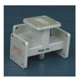
If another arm is added either to T-junction, then hybrid T-junction, is symmetrical about an imaginary plane bisecting arm3&4 and has very useful property. Magic Tee may be used in front end of the microwave receiver. The basic property in that arm3 and 4 are both connecting to arms1 and 2 but not to each other. This applies for dominant mode only, provided each arm is terminated at the correct load.
